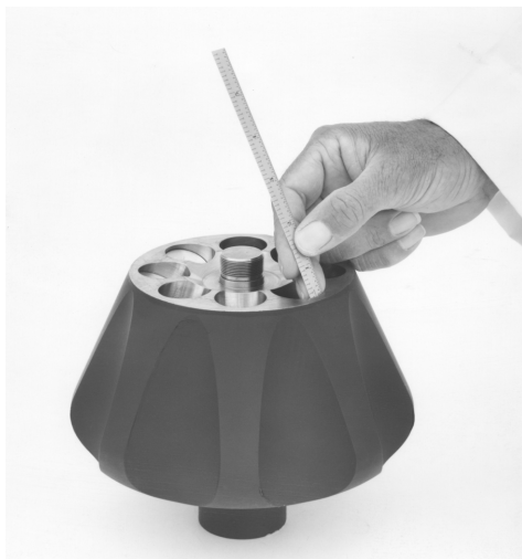
Figure 3 Measuring Distance from Cap to Rotor Tray
